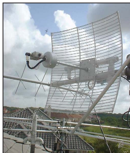
Fig 23.47 —K5OE's mesh modification of a MMDS dish antenna with helix CP feed and DEM preamp.
