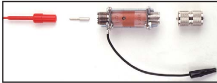
Fig 25.54 — A view showing the 10x multiplier with grabber, pin tip and a male UHF coupler that connects the multiplier to the RF probe.
