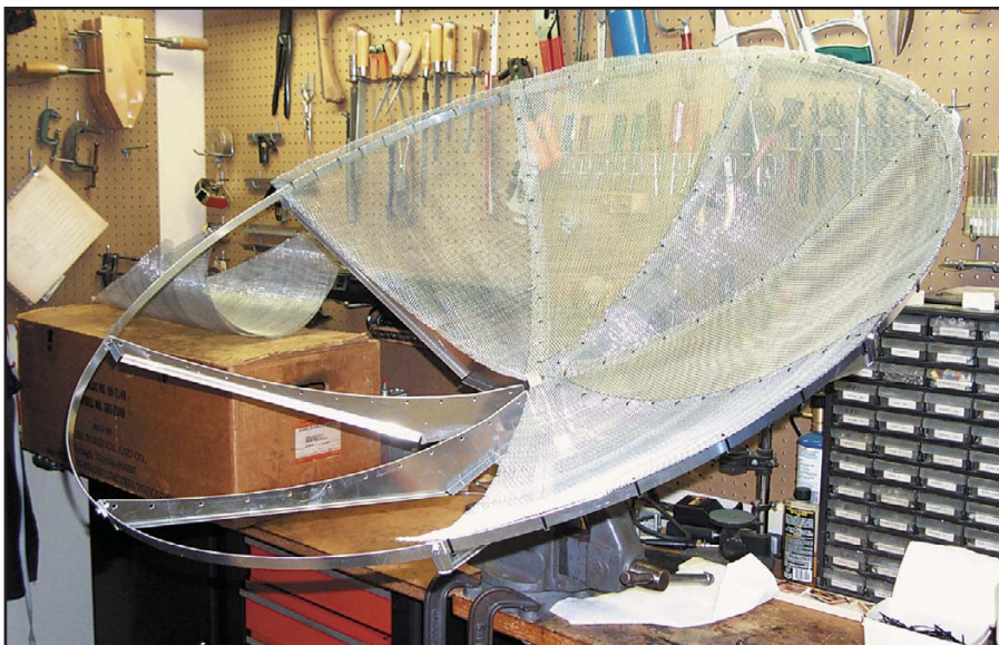
Fig 23.61—Dish antenna during assembly.
