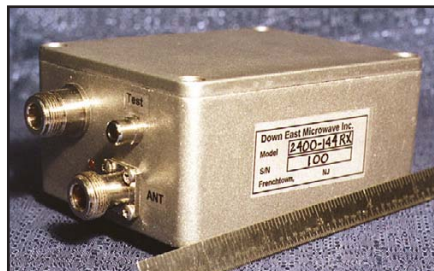
Fig 23.36 —This SSB Electronic unit (left) is one of several solutions for mast-mounted S-band receive converters. Other manufacturers, including Down East Microwave (top), have similar offerings.
