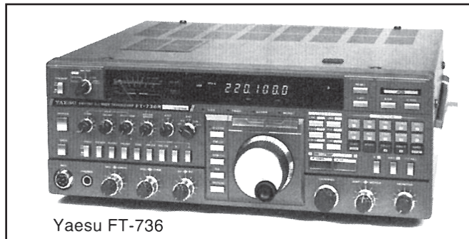
Fig 23.23 —The Yaesu FT-736R is a multi-mode transceiver for 2 m (144-148 MHz) and 70 cm (430-450 MHz). It can be used for full-duplex receiving and transmitting on Mode U/V and V/U. An optional 23-cm module covers 1230-1300 MHz (Mode L/U). Approximate power output: 20 W on 2 m and 70 cm, and 10 W on 23 cm.
