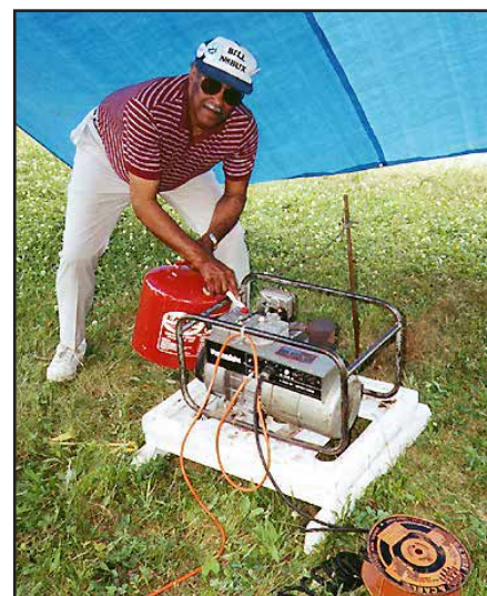
Fig 19.29 —Modern gasoline engine-powered generators offer considerable ac power output in a relatively compact and lightweight package.
