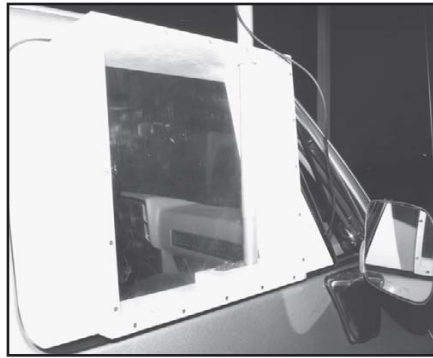
Fig 13.40 — A window box allows the navigator to turn a mast mounted antenna with ease while remaining dry and warm. No holes in the vehicle are needed with a properly designed window box.
