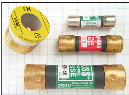
Fig 4.11 — These photos show examples of various styles of fuses. The ¼-inch-ruled graph paper background provides a size comparison.
