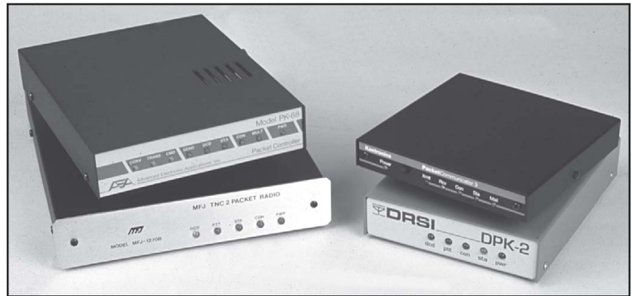
Fig 9.18—Four popular 1200 bit/s packet TNCs: (clockwise, from bottom left) the MFJ-1270C, AEA PK-88, Kantronics KPC-3 and the DRSI DPK-2.
