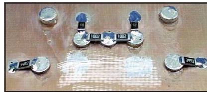
Fig F —SMT resistors soldered to base board of the Audio Amp in the beginning stages of assembly.
