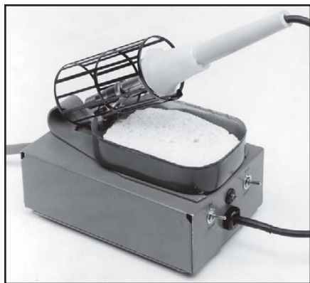
Fig 8.4—A compact assembly of commonly available items, this soldering station makes soldering easier. Miniature toggle switches are used because they are easy to operate.
