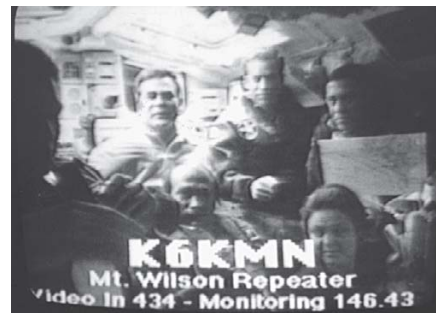
Fig 9.49 —A photo of an ATV image of the Space Shuttle interior with K6KMN's repeater ID overlaid. Automatic video overlay in the picture easily solves the 10-minute ID requirement for Space Shuttle retransmissions and other long transmissions.
