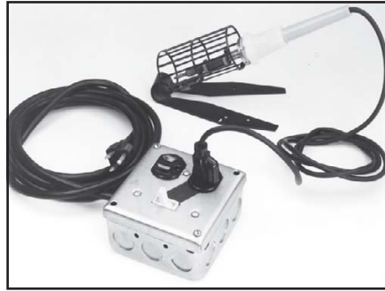
Fig 8.7—An incandescent-light dimmer controls soldering-iron tip temperature. Only one of the duplex outlets is connected through the dimmer.
