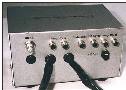
Fig 19.61 —A view of the rear panel of the main box of the Two-Radio Switchbox.
