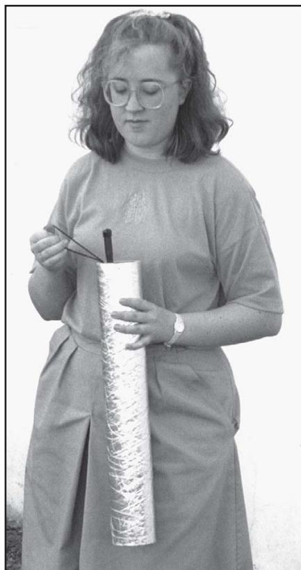
Fig 13.45 — The air attenuator for a VHF hand-held in use. Suspend the radio by the wrist strap or a string inside the tube.
