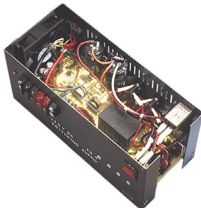
Fig 17.34 — Photo of the completed 13.8-V, 40-A switching supply built by WR1B.
