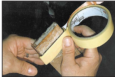
Fig 17.37 — Winding the foil tape tightly on the epoxy-coated-paper bobbin on the wooden block. The Mylar tape is unrolled and positioned over the foil layer as you wind. (Photo by Dan Wolfgang.)
