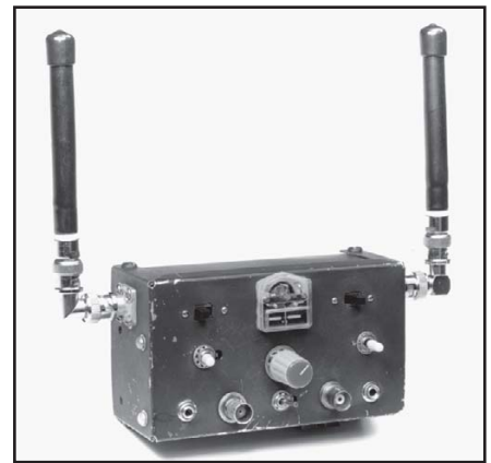
Fig 13.48 — Field version of the Simple Seeker with helix antennas.
