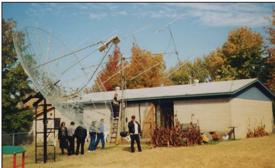
Fig 23.67 —Tommy Henderson, WD5AGO, pursues 144-MHz EME from his Tulsa, Oklahoma, QTH with this array. Local electronics students helped with construction.
