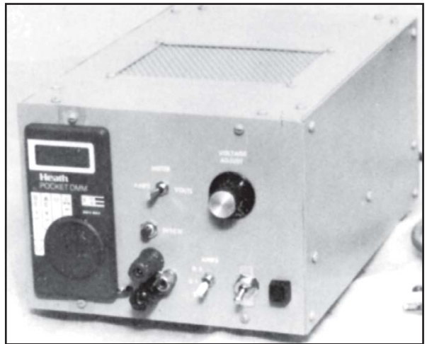
Fig 17.29 — An exterior view of the 2.5-A power supply. The DMM is mounted on the control panel as the output meter.
