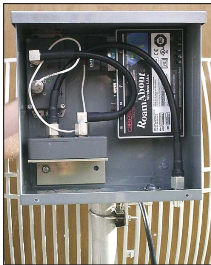
Fig 9.61—View of HSMM equipment (802.11b) inside an antenna-mounted NEMA-4 box. Mounting the equipment at the end of the dish antenna's pigtail significantly reduces feed line losses and greatly enhances the performance of the station. The box contains both a bridge, and a 500 mW bidirectional amplifier or BDA (lower left). Amplifier power is provided by the power insertion module seen in the upper left corner of the enclosure. (Photo: John Champa, K8OCL).
