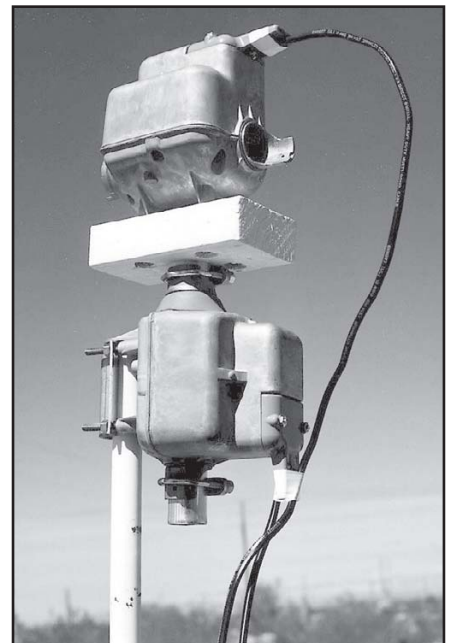
Fig 23.41—VE5FP has a solution for his Az-El rotators by bolting two of them together in his “An Inexpensive Az-El Rotator System,” QST, December 1998.
