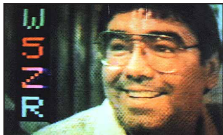
Fig 2.12 — An SSTV image as seen on a standard TV set using a digital scan converter.
