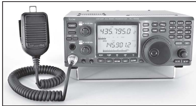
Fig 23.22 —ICOM’s IC-910H, a recent entry into the multi band VHF/UHF transceiver world, has an available 23-cm module.
