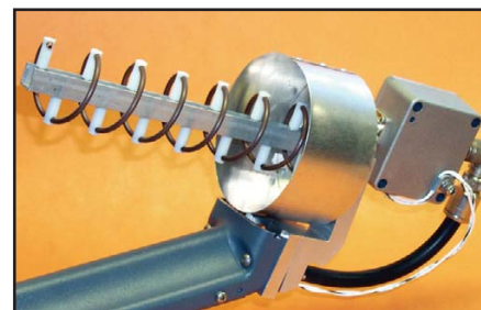
Fig 23.55—Seven-turn LHCP helix dish feed antenna with DEM preamp.
