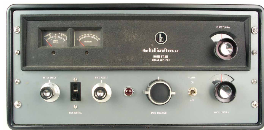
Fig 19.84—Typical of ham gear from the 1950s and early 1960s, this classic Hallicrafters HT-33B Linear Amplifier features a 117 V ac plate transformer. The magnetic circuit breaker on the front panel trips at a line current of 22 Amps! Many existing 110 to 120 V ac branch circuits would be unsuitable for such a load.
