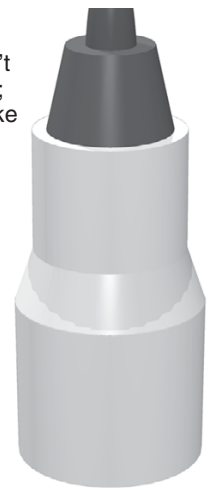
Fig A—Make a permanent marker into a specialized PC-board drawing tool. Simply press the marker point into a drilled hole to form a modified point as shown. More pressure produces a wider shoulder that makes larger pads on the PC board.
