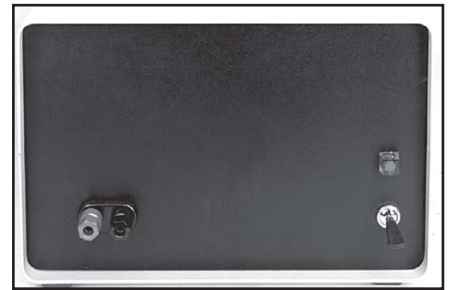
Fig 17.44 — The front panel of the 28-V power supply sports only a power switch, pilot lamp and binding posts for the voltage output. There is room for a voltmeter, should another builder desire one.
