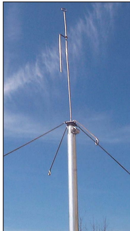
Fig 22.99 — WA3WMG's whip can be used to make a dual-band groundplane antenna. Separate radials for 2-m and 70-cm simplifies tuning. [Photo by K8CH]
