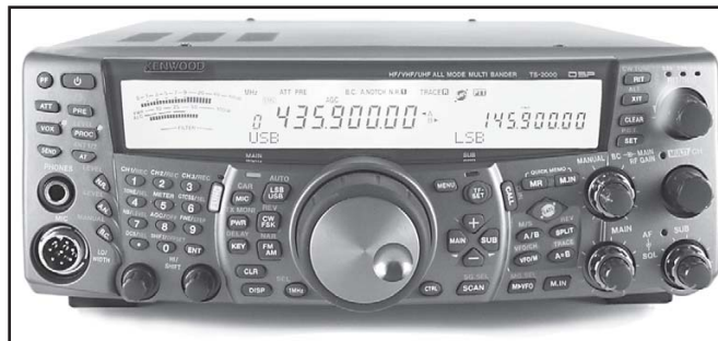
Fig 23.24 —Kenwood’s TS-2000 is an all-band, multi-mode transceiver that covers HF, 6 m, 2 m, and 70 cm. A 23-cm (1240-1300 MHz) module is optional. Typical power output is 35-45 W on 144 MHz, 30-40 W on 430 MHz and 10 W on 1240 MHz.
