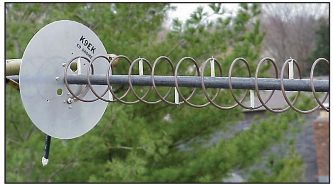
Fig 23.43 —This L-band helix antenna was designed to be home-brewed without any special tools or shop equipment. It is mounted on a 4-foot-long fiberglass tube.
