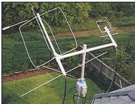
Fig 23.14 —Jerry Brown, K5OE, uses his Texas Potato Masher antennas for LEO satellite operations.
