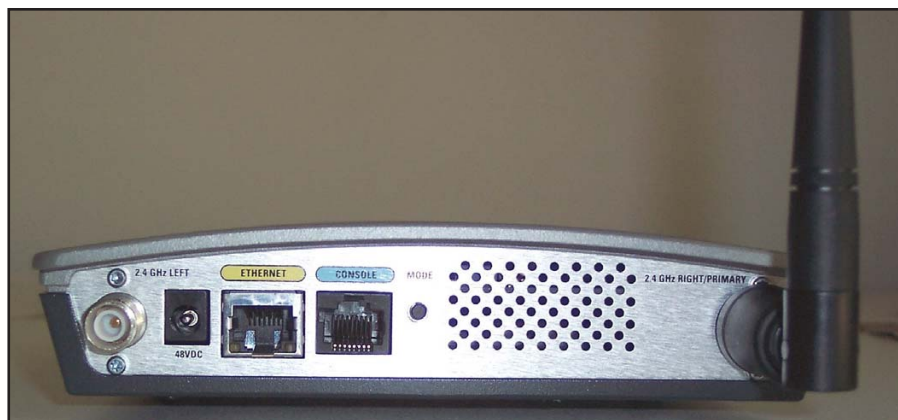
Fig 9.60 —Back panel of a typical HSMM-style repeater. This device is known commercially as a wireless access point (AP). It is essentially a computer wireless network hub to enable multiple radio stations to share the various resources of the network. This particular model is a Cisco Model 1200. Note that the left, or secondary antenna's rubber duck has been removed from the TNC connector to show that the connector is of the reverse polarity (RP) type. This is designated as a female TNC/RP connector. Manufacturers of 802.11 gear typically install a RP-type of some type connector to prevent FCC Part 15 unlicensed users from employing their equipment in a non-certified manner. Of course, this is not an issue for licensed Part 97 users, however as in this case, a male RP-type plug will be required in order to connect the device to an outside antenna. The provision of a secondary antenna is to provide space diversity, which helps reduce the negative impact of multipath propagation of the radio signals. The secondary antenna may be ignored when connecting the primary antenna to a single outside antenna, especially if it is a highly directive antenna, which would help reduce multipath effects. (Photo: John Champa, K8OCL).
