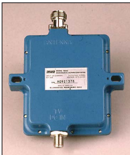
Fig 23.35 —S-band converter that was available from Drake, and easily modified for satellite service.
