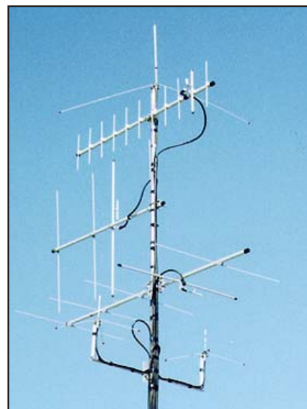
Fig 23.15 —Simple ground plane and Yagi antennas can be used for low-Earth-orbit (LEO) satellite contacts.
