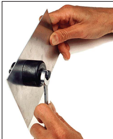
Fig 8.3 —A socket punch is used to easily punch a hole in sheet metal.
