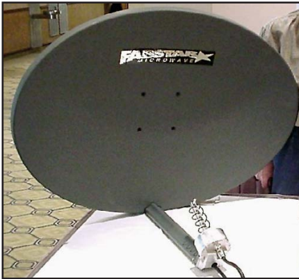
Fig 23.50 —PrimeStar offset-fed dish with WD4FAB’s helix-feed antenna. N0NSV was so pleased with the modification that he renamed the dish “FABStar,” and made a new label!
