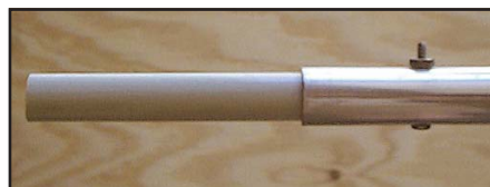
Fig 22.55 — The HVD base insulator is a 1-ft length of 0.75-inch fiberglass rod.
