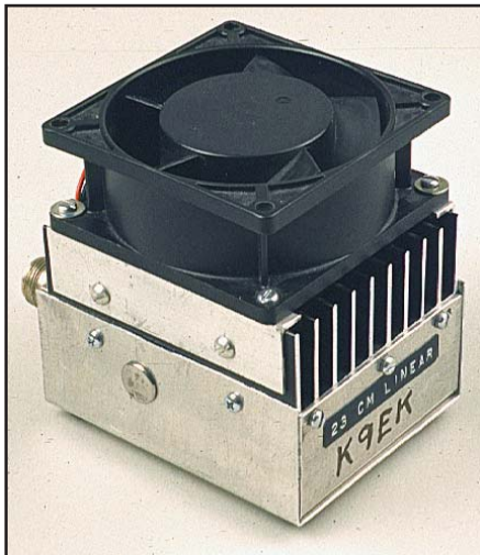
Fig 23.27 —The matching brick amplifier can be mounted on the counterbalance side of the Helix antenna boom.
