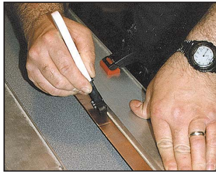
Fig 17.36 — Larry Wolfgang, WR1B, using a 4-foot straightedge designed as a guide for hand-held circular saws to clamp the copper-foil tape to a board on a tabletop. After carefully measuring to ensure a uniform 22-mm width, he cut the foil tape using a Fiskars rotary cutter. Be careful to keep the cutter wheel against the straightedge for the entire length. Move the tape in 4-foot intervals to cut the entire length. (Photo by Dan Wolfgang.)
