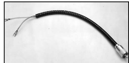
Fig 21.16—W2DU bead balun consisting of 50 FB-73-2401 ferrite beads over a length of RG-303 coax. See text for details.
