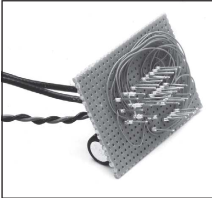
Fig 8.17—The audio amplifier built using wire-wrap techniques.
