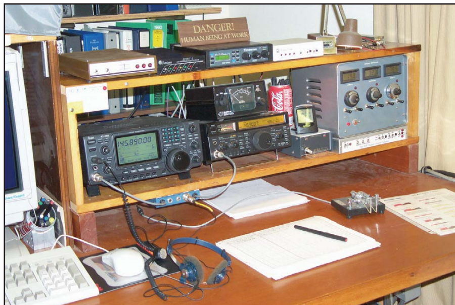
Fig 23.20 —WD4FAB's station is typical of a full-featured HF and satellite operation. On the bottom row, L-R are: IC-746 HF to 2 meter transceiver, IC-821H VHF-UHF multimode transceiver topped by a home-brew power meter, KLM 1200GU 1.2-GHz transverter, home-brew multi-antenna rotator controller on top of the station accessory control box. On the top row, L-R are: G3RUH AO-13 Telemetry Demodulator, PacComm SPIRIT2 high performance packet controller, Timewave DSP-599zx audio DSP unit for the VHF-microwave operations through the IC-821H and the TAPR EasyTrak antenna command unit for interfacing the computer tracking to the antenna controller.
